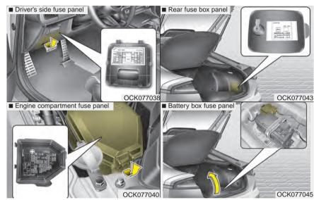
Inside the fuse/relay panel covers, you can find the fuse/relay label describing fuse/relay name and capacity.
