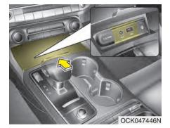
You can use an AUX port to connect audio devices and an USB port to plug in an USB or iPod®.
