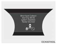
The message will appear to notify the driver if there are foreign substances on the surface or inside the rear bumper or it is hot near the rear bumper. The light on the switch and the system will be turned off automatically.
