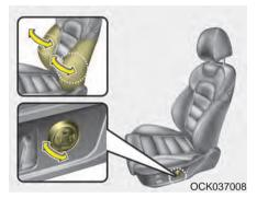
Turn the adjustment switch clockwise, the right/left seatback bolsters will be adjusted inward. Turn the switch counterclockwise, the seatback bolster will be adjusted outward.
