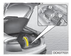
The battery is in the luggage room. When replacing the battery, disconnect the negative (-) cable (1) and remove the positive (+) battery fuse box (2). Remove the battery mounting bracket (3).
