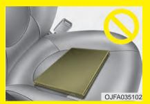
Do not place electronic devices such as laptops, DVD player, or conductive materials such as water bottles on the passenger seat.
