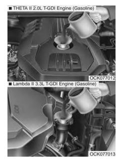
If it is near or at L, add enough oil to bring the level to F. **Do not overfill.**
