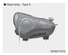
If the position lamp + DRL (LED) (1) does not operate, have the vehicle checked by an authorized Kia dealer.
