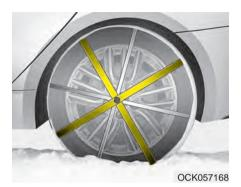
Since the sidewalls on some radial tires are thinner than other types of tires, they may be damaged by mounting certain types of tire chains on them. Therefore, the use of snow tires is recommended instead of tire chains. Do not mount tire chains on vehicles equipped with aluminum wheels; if unavoidable, use AutoSock (fabric snow chain). Install the tire chain after reviewing the instructions provided with the tire chains.
