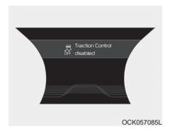
To cancel ESC operation, press the ESC OFF button (ESC OFF \$\frac{1}{20}\$) shortly (ESC OFF indicator light (ESC OFF \$\frac{1}{20}\$) illuminates). At this state, the engine control function does not operate. It means the traction control function does not operate. Brake control function only operates.
