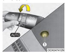
Dynamic Bending Light (DBL) uses the steering angle and vehicle speed, to keep your field of vision wide by swiveling and leveling the headlamp. Change the switch to the AUTO position when the engine is running. The dynamic Bending Light (DBL) will operate when the headlamp is ON. To turn off the DBL, change the switch to other positions. After turning the DBL off, headlamp swiveling no longer occurs, but leveling operates continuously.
