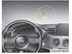
The head up display is a transparent display which projects a shadow of some information of the instrument cluster and navigation on the windshield glass.
