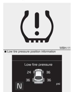
When the tire pressure monitoring system warning indicators are illuminated, one or more of your tires is significantly under-inflated.
