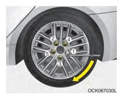
Position the wrench as shown in the drawing and tighten the wheel nuts. Be sure the socket is seated completely over the nut. Do not stand on the wrench handle or use an extension pipe over the wrench handle. Go around the wheel, tightening every nut following the numerical sequence shown in the image until they are all tight. Double-check each nut for tightness. After changing wheels, have an authorized Kia dealer tighten the wheel nuts to their proper torque as soon as possible.
