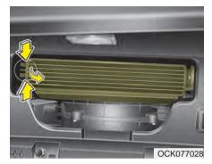
3. Remove the climate control air filter cover while pressing the lock on the left side of the cover.
