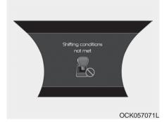
The warning message appears on the LCD display, when engine RPM is too high, or when driving speed is too fast to shift the gear.
