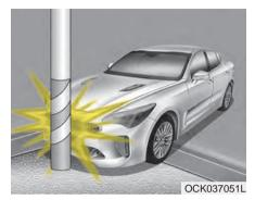
Air bags may not inflate if the vehicle collides with objects such as utility poles or trees, where the point of impact is concentrated to one area and the full force of the impact is not delivered to the sensors.
