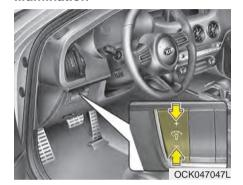
The brightness of the instrument panel illumination is changed by pressing the illumination control button ("+" or "-") when the Engine Start/Stop button is ON, or the taillights are turned on.
