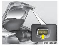
• Press the power liftgate close button for approximately one second when the liftgate is opened. The liftgate will close and lock
