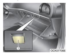
If the glove box lamp (LED) (1), does not operate, have the vehicle checked by an authorized Kia dealer. The LED lamps cannot be replaced as a single unit because it is an integrated unit. The LED lamps has to be
