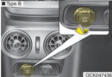
The power outlet is designed to provide power for mobile devices.
