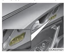
Driving Position Memory System is the facility that enables driver's seat, steering wheel, exterior mirrors, cluster and head-up display (HUD) to be controlled with a simple button operation, which allows a driver to recall memorized driving positions and automatically control them. Driver's seat/ Steering Wheel/ Exterior mirrors: location Cluster: Brightness of lighting
