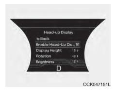
The HUD display will be activated or deactivated in user setting mode while engine is ON.
