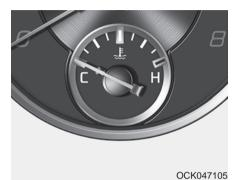
This gauge indicates the temperature of the engine coolant when the Engine Start/Stop button is ON.
