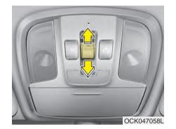
To open the sunshade Push the sunroof control lever backward to the 1st detent position.
