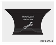
The warning message appears on the LCD display, when the transmission or the shift lever does not properly operate in the P (Park) position. In this case, we recommend you to immediately have the vehicle inspected by an authorized Kia dealer
