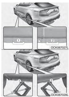
7. Place the jack at the front (1) or rear (2) jacking position closest to the tire you are changing. Place the jack at the designated locations under the frame. The jacking positions are plates welded to the frame with two tabs and a raised dot to line up with the jack.
