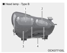
If the Low/High beam lamp(1,2), Front turn signal lamp(3), Day time running lamp/Position lamp(4), Side marker (5) does not operate, have the vehicle checked by an authorized Kia dealer.
