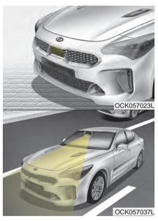
In order for the FCA system to operate properly, always make sure the sensor or sensor cover is clean and free of dirt, snow, and debris. Dirt, snow, or foreign substances on the lens may adversely affect the sensing performance of the sensor.
