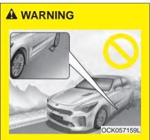
Never start or run the engine while an AWD vehicle is raised on a jack. The vehicle can slip or roll off of a jack causing serious injury or death to you or those nearby.
