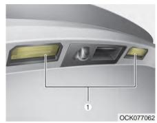
If the license plate lamp (LED) (1), does not operate, have the vehicle checked by an authorized Kia dealer. The LED lamps cannot be replaced as a single unit because it is an integrated unit. The LED lamps has to be replaced with the unit.
