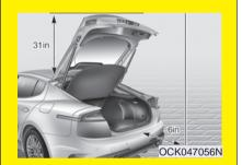
Make sure that there are no people or objects in the path of the power liftgate (or smart liftgate) prior to use. Serious injury, damage to the vehicle or damage to surrounding objects may result if contact with the power liftgate (or smart liftgate) occurs.
