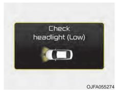
This warning message illuminates if there is a malfunction (burned-out bulb except LED lamp or circuit malfunction) with the headlamp. In this case, have your vehicle inspected by an authorized Kia dealer.
