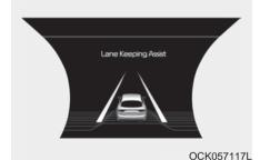
If the speed of the vehicle is over 40 mph (64 km/h) and the system detects lane markers, the color changes from gray to white. When the conditions below are met, LKA SYSTEM will be enable to assist steering.
