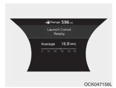
Press the brake firmly with your left foot in transmission D mode, while pressing the accelerator pedal down fully with your right foot. Then, the Launch Control Ready (1) will be in place.
