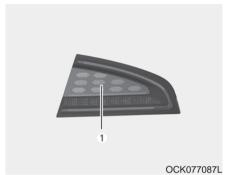
If the rear turn signal lamp (LED) (1), does not operate, have the vehicle checked by an authorized Kia dealer. The LED lamps cannot be replaced as a single unit because it is an integrated unit. The LED lamps has to be replaced with the unit.
