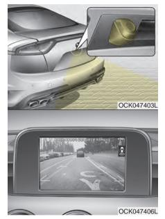
The rearview camera will activate with the ignition switch ON, engine ON and the shift lever in the R (Reverse) position.
