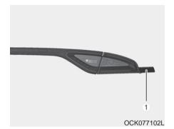
If the rear side marker (LED) (1), does not operate, have the vehicle checked by an authorized Kia dealer. The LED lamps cannot be replaced as a single unit because it is an integrated unit. The LED lamps has to be replaced with the unit.
