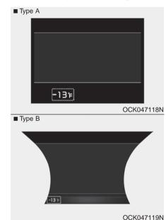
This gauge indicates the current outside air temperatures by 1°F (1°C).
