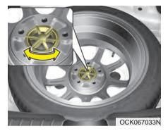
Turn the tire hold-down wing bolt counterclockwise.
