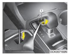
You can move the shift lever, when the battery is discharged. However, it will not change the gear from P (Parking) to N (Neutral) or others.
