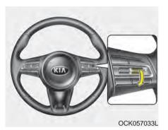
Move the lever down (to SET-), and release it at the desired speed. The cruise indicator and set speed on the LCD screen will illuminate. Release the accelerator at the same time. The desired speed will automatically be maintained.
