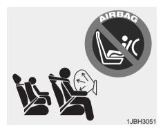
Never place a rear-facing child restraint in the front passenger's seat. If the air bag deploys, it would impact the rear-facing child restraint, causing serious or fatal injury.
