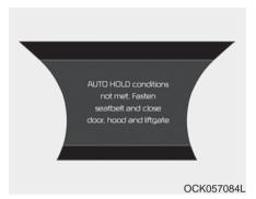
When you press the [AUTO HOLD] switch, if the driver's door, engine hood are not closed or the driver's seat belt is unfastened, a warning will sound and a message will appear on the LCD display. At this moment, press the [AUTO HOLD] button after closing the driver's door, engine hood and fastening the seat belt.
