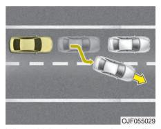
When driving in stop-and-go traffic, and a stopped vehicle in front of you erges out of the lane, the FCA system may not immediately detect the new vehicle that is now in front of you. In this case, you must maintain a safe braking distance, and if necessary, depress the brake pedal to reduce your driving speed in order to maintain a safe distance.
