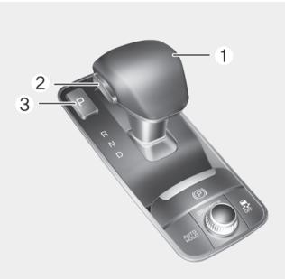
When you move the shift lever (1), depress the brake pedal while pressing the UNLOCK button (2).
