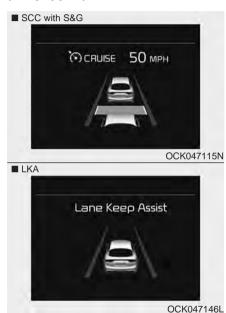
This mode displays the state of the Smart Cruise Control with Stop & Go and Lane Keeping Assist (LKA).
