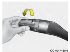
When the light switch is in the parking light position, the tail, license and instrument panel lights will turn ON.
