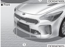
The parking assist system assists the driver during movement of the vehicle by chiming if any object is sensed within the distance of 39 in. (100 cm) in front and 47 in. (120 cm) behind the vehicle
