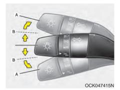
The ignition switch must be on for the turn signals to function. To turn on the turn signals, move the lever up or down (A). The green arrow indicators on the instrument panel indicate which turn signal is operating.
