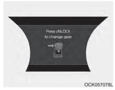
The warning message appears on the LCD display, when the [UNLOCK] button is not pressed while shifting the gear. We recommend you to press the [UNLOCK] button and then shift the gear.
