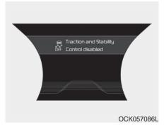
To cancel ESC operation, press the ESC OFF button (ESC OFF 3) for more than 3 seconds. ESC OFF indicator light (ESC OFF 3) illuminates and ESC OFF warning chime will sound. At this state, the engine control function and brake control function do not operate. It means the car stability control function does not operate any more.
